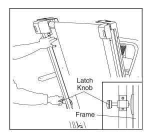
Hold the metal frame firmly with both hands, and lower it to the floor. CAUTION: To decrease the possibility of injury, do not lower the frame by gripping only the plastic foot rails; do not drop the frame to the floor. Make sure to bend your legs and keep your back straight.
